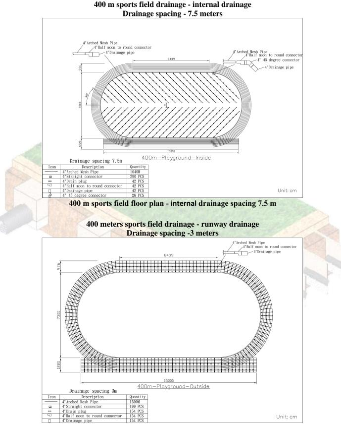
400 m sports field floor plan - runway drainage spacing 3.0 m
