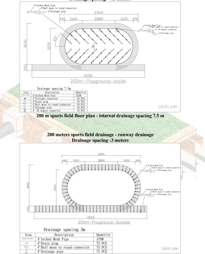
200 m sports field floor plan - runway drainage spacing 3.0 m
